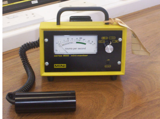
Figure 3.2: How can we find the true count rate of a Geiger counter which suffers from dead-time.
