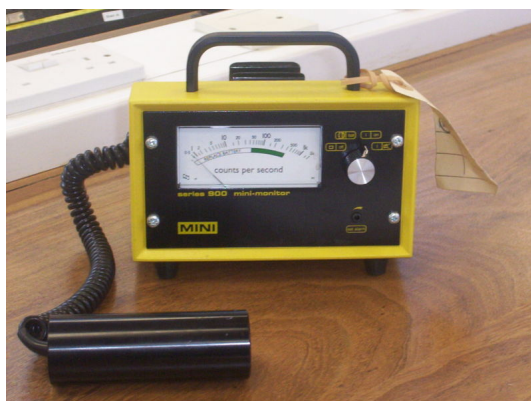
Figure 9.13: How can we find the true count rate of a Geiger counter which suffers from dead-time.
